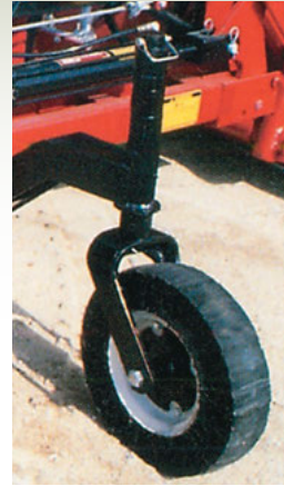
The optional, adjustable tailwheel provides extra support for the main beam — a real plus when working on rugged terrain.
