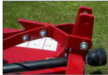
Floating Hitch for uneven terrain
