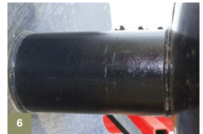
[1] Standard Rigid Hanger [2] Blade Scrapers [3] Adjustable Gang Angle [4] Positive Depth Control [5] Removable Spindle Axles [6] Steel Fabricated Spools [7] Large gang shaft [8] Furrow filler blade
