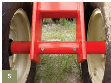
[1] Standard Rigid Hanger [2] Blade Scrapers [3] Adjustable Gang Angle [4] Positive Depth Control [5] Removable Spindle Axles [6] Steel Fabricated Spools [7] Large gang shaft [8] Furrow filler blade
