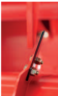
A patented system - the knives pass the fixed comb on alternative sides for a more even cut.
