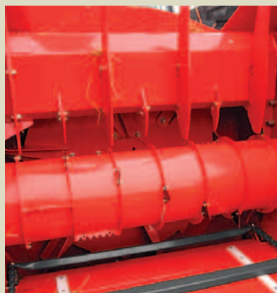
The drum-comb combination is designed for shredding straw bales in all formats.
