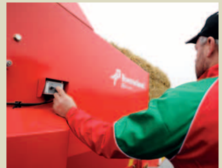
Operating both tailgate as well as floor chain in a safe distance from the moving parts by using the remote control placed on the side of the 853 Pro and 856 Pro
