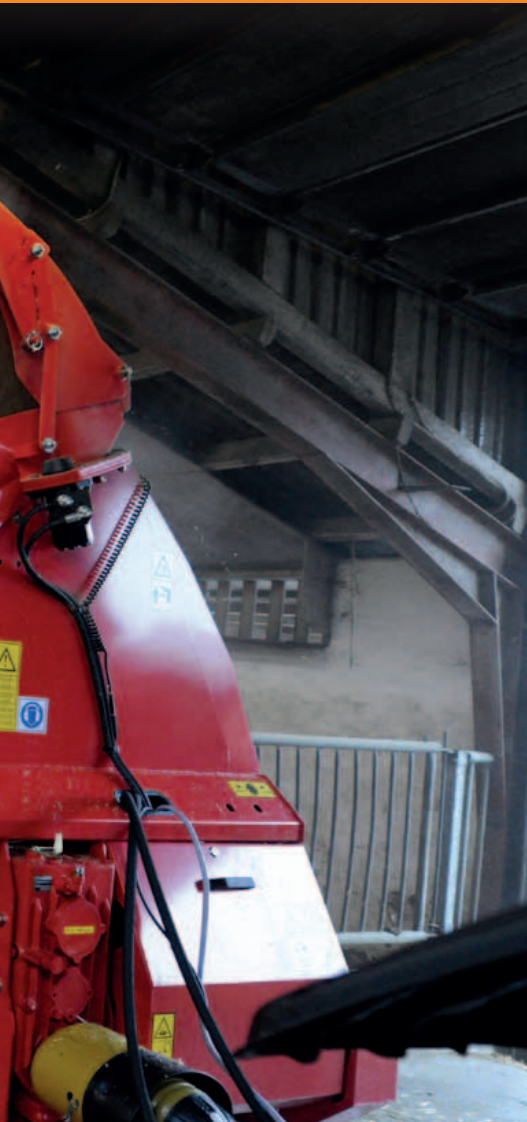
DFCS engaged to reduce the risk of blockages during loading and flywheel start up.
