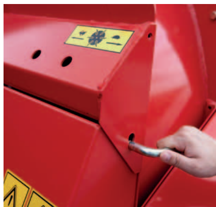
Easy shifting from from bedding to feeding on the 2-speed gearbox.
