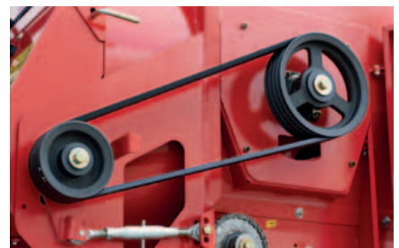
V-belt drive - low maintenance and quiet drive of the drum.
