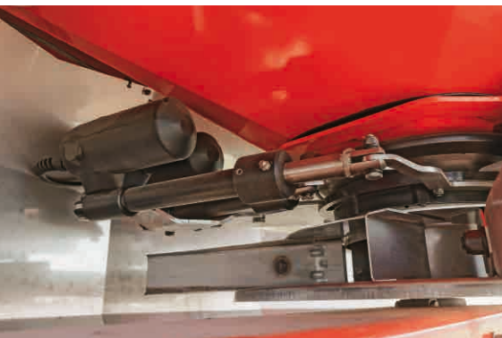
Two actuators on each dosing unit to control the discharge point and application rate
