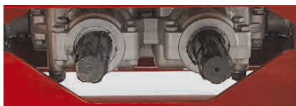
Centre gear box with 2 input shafts for high and low disc speed settings
