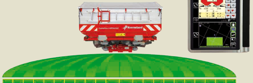
Example: Full spreading width of 54m with 24 sections
