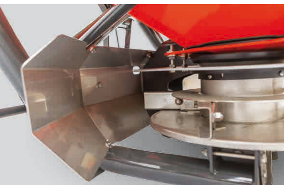
4 detachable vanes per disc determine the working width
