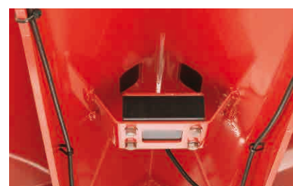
1 x Reference sensor, unique to Kverneland Exacta
