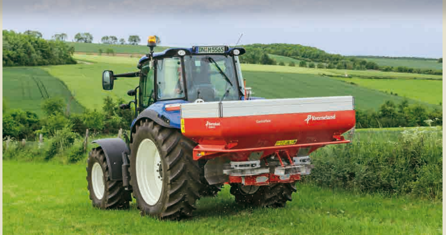
Border spreading using the border spreading plate (available as manual or hydraulic version)
