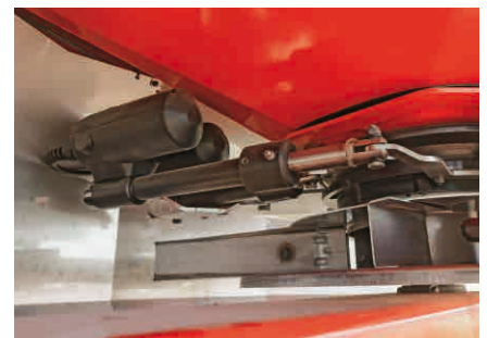
Two actuators on each dosing unit to control the discharge point and application rate.
