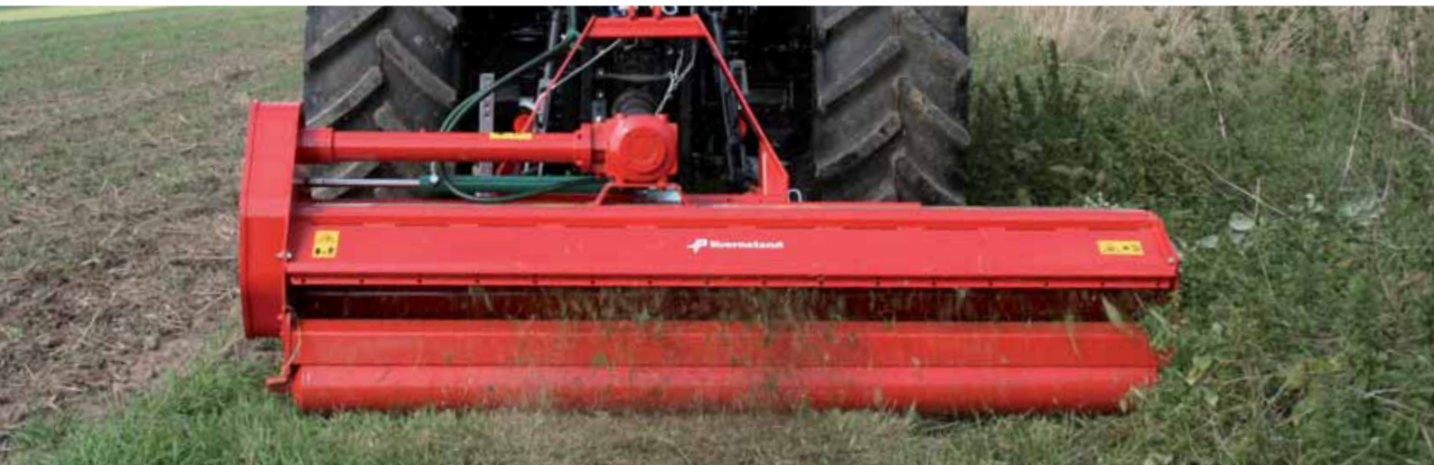
Double skin as standard equipment as it is an integral part of the frame. Standard thickness of 4mm.
