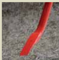
"C" Tine with standard reversible plough point.
