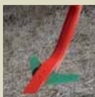
Standard reversible point in combination with 30cm wing share for shallow working.
