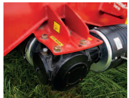
Two speed gearbox – switched by turning the main gearbox 180°.
