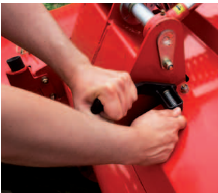
The conditioner plate can be set in 3 positions according to the required conditioner effect.
