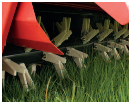
Rigid nylon tines provide aggressive conditioning.
