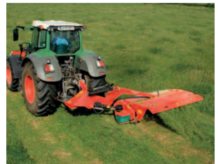
The centre suspended design ensures excellent ground adaptation.
