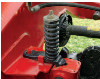
BreakBack system for optimal protection of the cutterbar.
