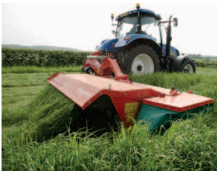
Kverneland Taarup cutterbar for improved cutting performance.
