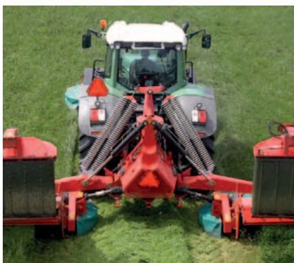
4 large springs ensure even flotation and cutting height.
