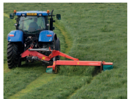
The centre suspended design ensures excellent ground adaptation.
