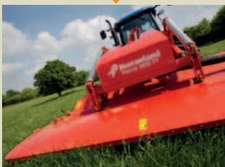
Suspension springs moved further outwards for better side stability and even ground pressure.
