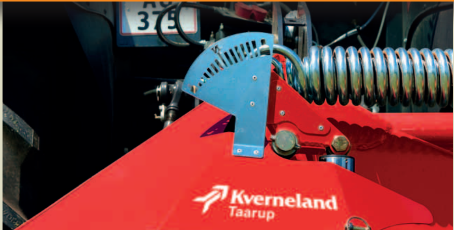
Hydraulic on-the-go setting of ground pressure.
