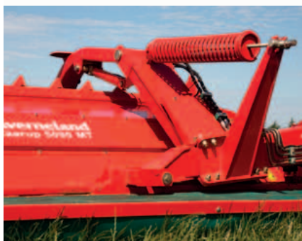
The Kverneland NonStop Taarup BX-Belt system, with individual BreakBack of each rear mower.
