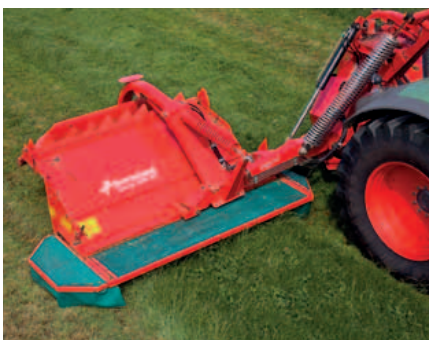
The centre suspension of the two rear mowing units provides excellent ground following.
