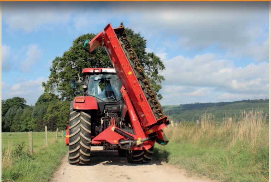
Kverneland Taarup 3200 MN/MR series machines are folded into a 125° vertical transport position using a hydraulic cylinder.
