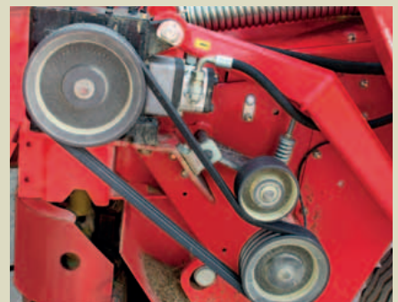
Adjustable rotor speed enables fuel saving and preservation of crop.
