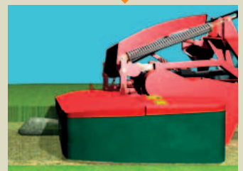
ActiveLift system to protect the cutterbar against foreign obstacles.
