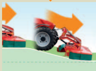
Mower reacts instantly to uneven ground contours and can move 250mm down and 450mm up.
