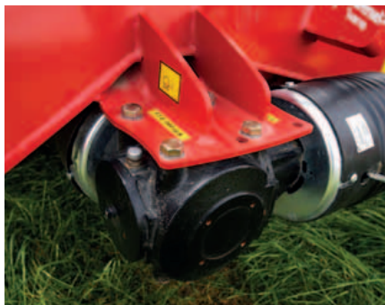
2-Speed gearbox – switched by turning the main gearbox 180°.
