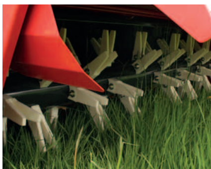
Rigid nylon tines provide aggressive conditioning.
