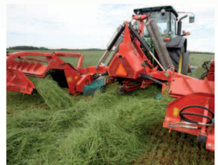
Three in one, 9.00m grass into one swath.
