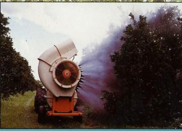
FAN, Mounted on a position above the conventional. It has nylon blades, resists chemicals action and requires low start torque. Its great air volume makes the chemicals penetrate the tree easily
