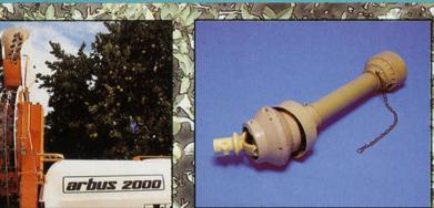
WIDE ANGLE CV JOINT SHAFT. Permits to make turns of up to 75° without disengaging the PTO.
