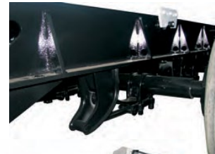
HD Spring Suspension (Hiway Commercial)
