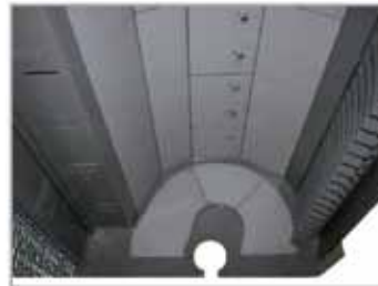
The internal protections of the machine are in HARDOX® steel, fully and easily interchangeable, ensuring a greater resistance to wear and reducing maintenance costs
