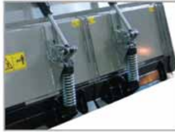
Rear hydraulic protection/grader flap to level the output material
