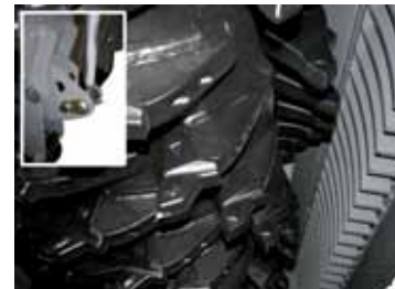
The adjustable grid on the rear hood is independent from the hood in order to work also on wet material (setting slots in the detail)
