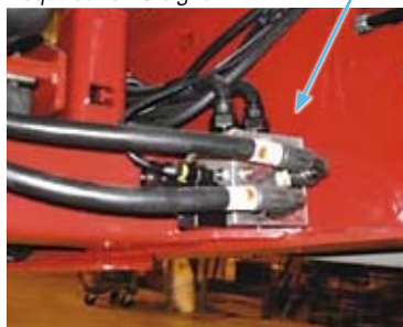
Optional bypass valve Required for LS signal
