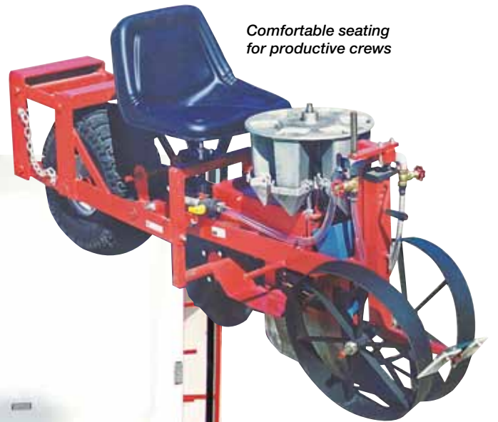
Rear jack allows quick adjustment of planting depth in the field
