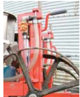
Rear jack allows quick adjustment of planting depth in the field
