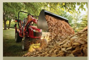
Our powerful front-end loaders with dual bucket cylinders maintain an even force across the bucket to keep it from getting out of line.
