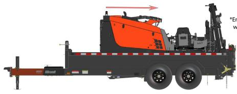
\*Ensure to park at the very back of the box when hauling a machine rear facing.
