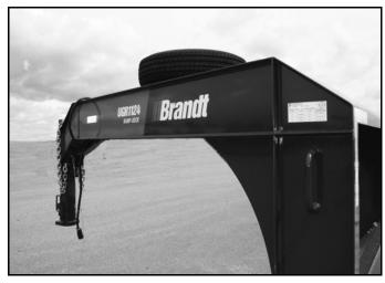
FIG. 4-10. Trailer with Gooseneck Coupler
