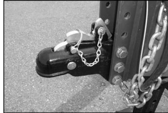
FIG. 4-2. Trailer with Ball Hitch Coupler
