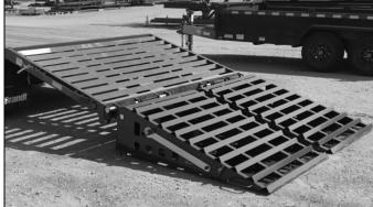
FIG. 5-3. Ramp Storage Position
