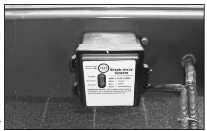
FIG. 4-7. Breakaway Brake Controller
