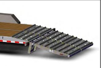
FIG. 5-2. Ramps in Storage Position and Working Position
