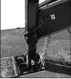
FIG. 4-17. Breakaway Brake System
