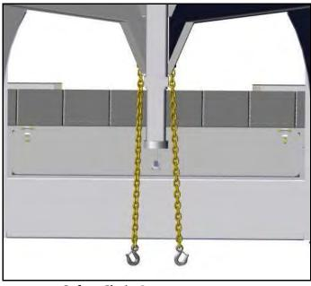
FIG. 4-16. Safety Chain Arrangement
