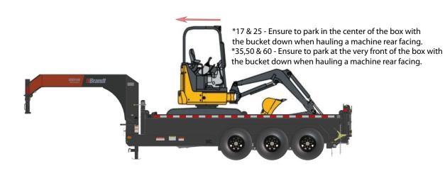
The following list details whether the specified size of Excavator will fit the trailer orientation.
