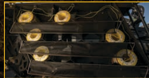
30-ball twine storage protected by a one-piece sealed shield to reduce crop buildup.
