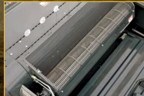
Hydraulically driven transverse knotter fan boosts efficiency by keeping trash buildup to a minimum, increasing overall reliability.
