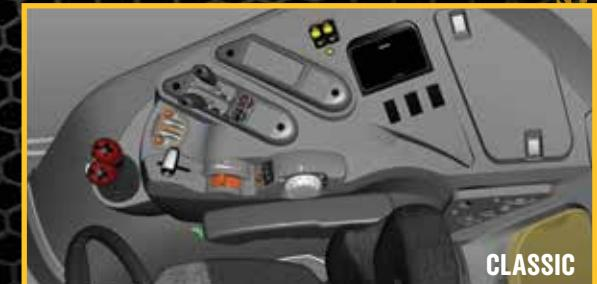
*Familiar layout ergonomically places T-handle transmission lever and hydraulic controls within easy reach on ride-side console alongside PTO and three-point hitch controls.*
