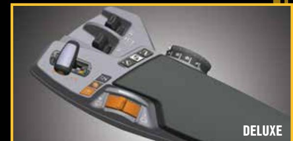
*Short control armrest features T-handle transmission and fingertip controls for hydraulic remotes, three-point hitch, engine speed and headland, throttle and Power Management.*
