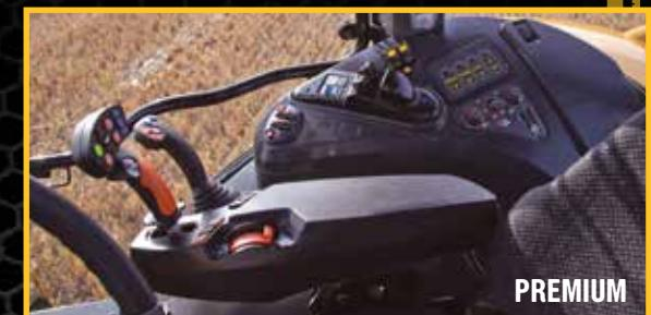
*Armrest with Multicontroller and Multifunction joystick for thumb and fingertip control of forward/reverse shuttling, PTO, programmable hydraulic functions, engine and cruise speeds.*
