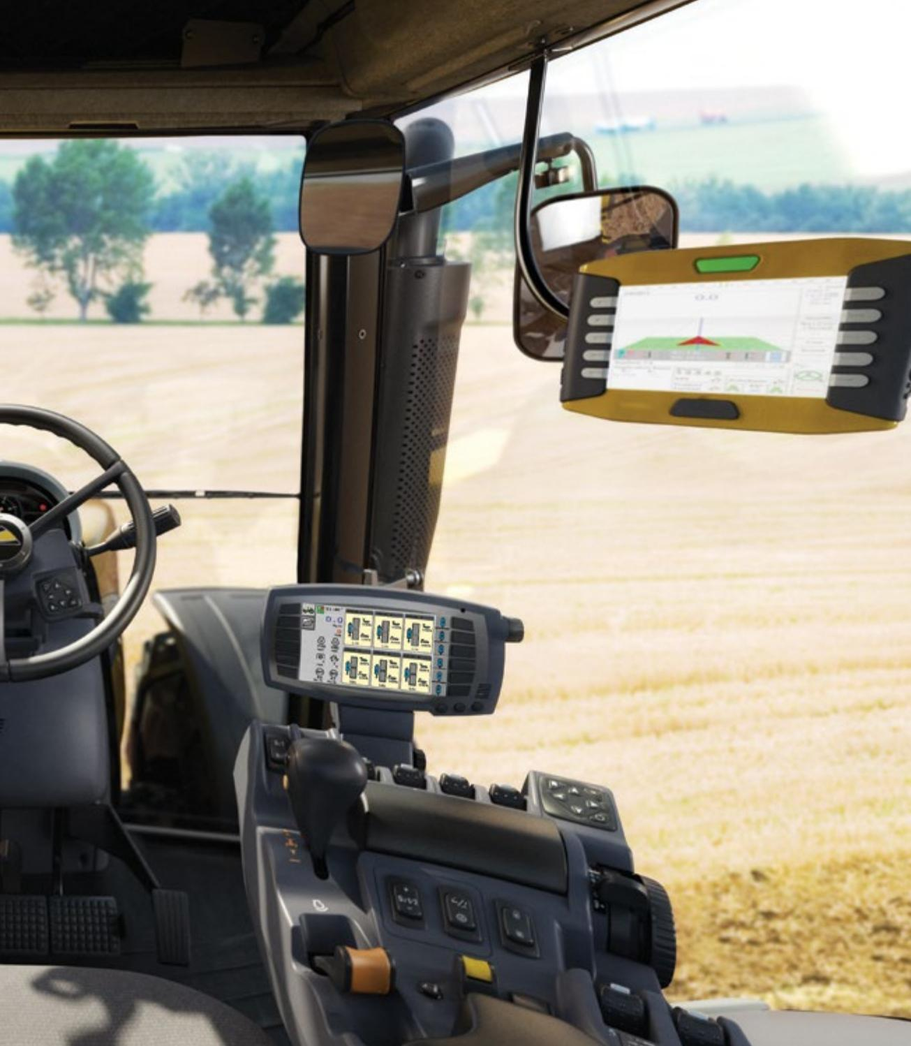
The intuitive and ergonomic design of the Tractor Management Center (TMC) puts all key functions — including six hydraulic control valves — at your fingertips.
