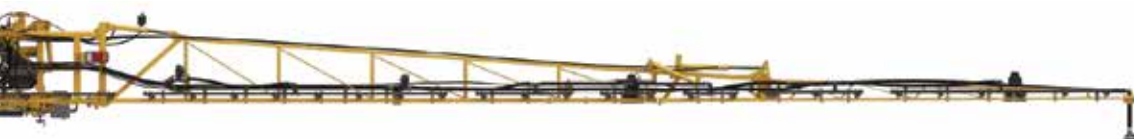
Boom Length 90 ft. (27 m), with 19-ft. (5.7 m) tip and full-boom breakaway
