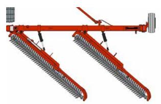
Adjust tine angle from 25° to 40° depending on field conditions and preference.
