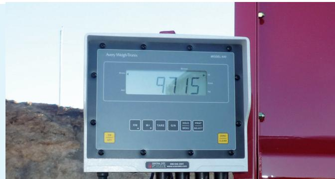
Scaled models come with 4 load cells and a large monitor that can be adjusted for viewing while loading from either side.
