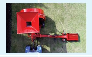
1016T fills 10' bags at up to 18,000 bushels per hour and requires a tractor with just 80 horsepower and 20 gallons-per-minute hydraulic capacity. Once the grain bags have been filled the innovative folding design makes the RGB 1016T easy to maneuver on roads, around bags, and in farm yards or storage sheds.
