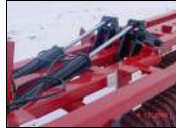
Rugged 4 beam main wing section w/two cylinders.
