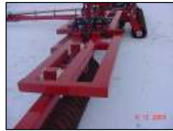
3 beam outerwing section w/two cylinders, each packer gang oscillates on centre pin and plastic wear plates.
