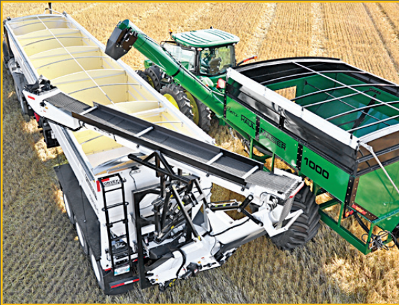
Conveyor swings out to load rear compartments.
