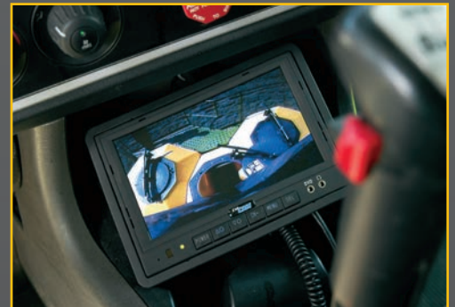
Positioning Camera. Equipped with microphone and in-cab monitor with speaker
