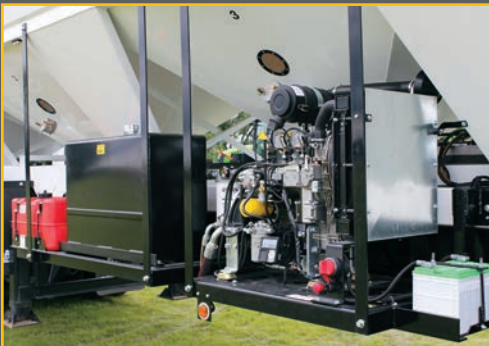
Self contained power pack. Gas or Diesel
