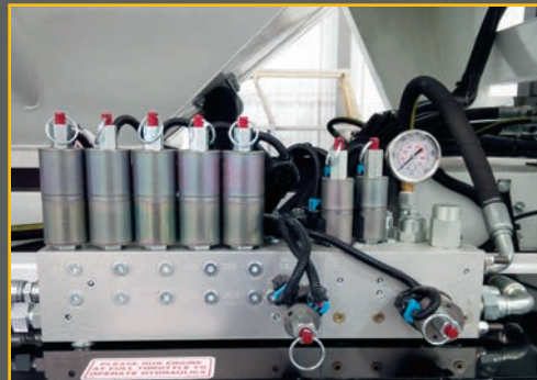
All aluminum anodized control valves
