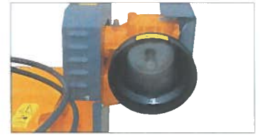
Gearbox unit outside the transmission cover (more offset and less PTO angle).
