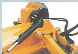
Rotation joint on self lubricating bushing
