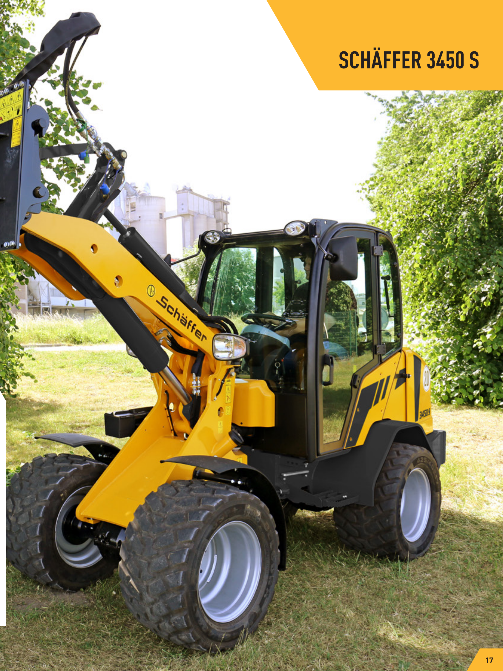
The 3450 S can move pallets weighing 2.0 tonnes. A narrow and very low front end optimises the driver's view of the attachment.
