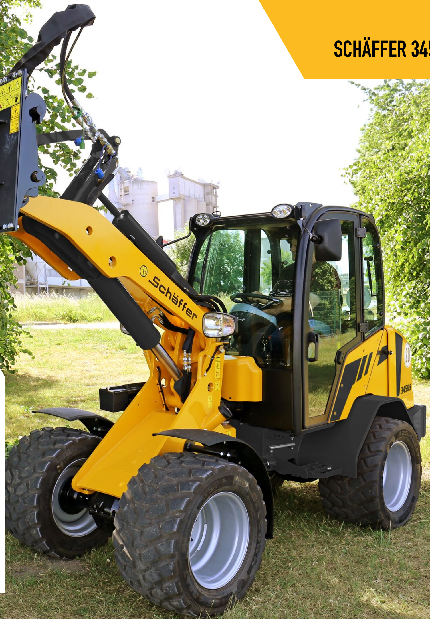
The 3450S can move pallets weighing 2.0 tonnes. A narrow and very low front end optimises the driver's view of the attachment.
