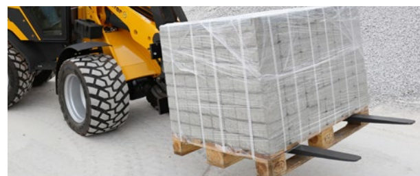
The 3450S can move pallets weighing 2.0 tonnes. A narrow and very low front end optimises the driver's view of the attachment.
