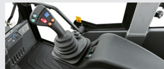
Arm-rest and joystick form a unit with the seat and accept all movements of the seat. This keeps the driver comfortable even on long working days.
