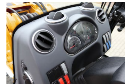
Additional, larger air outlets for perfect air circulation/ optimised range of switches
