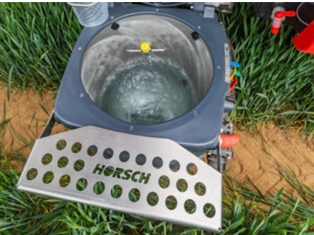
13.7 gal stainless steel induction hopper incl. additional shock nozzle
