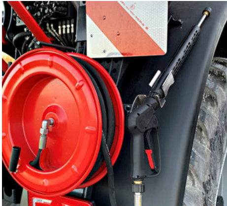
Hydraulically operated high-pressure cleaner
