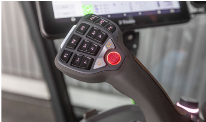
Ergonomic control lever with multiply assignable buttons
