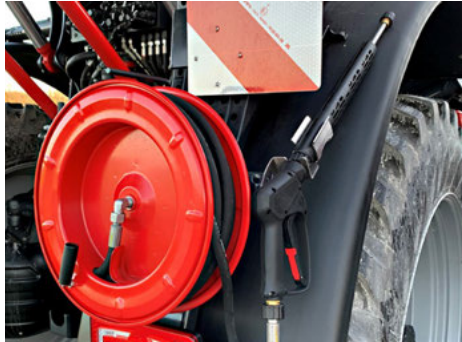
Hydraulically operated high-pressure cleaner
