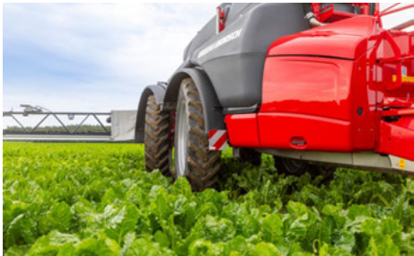
Active steering of both axles is integrated in the machine software
