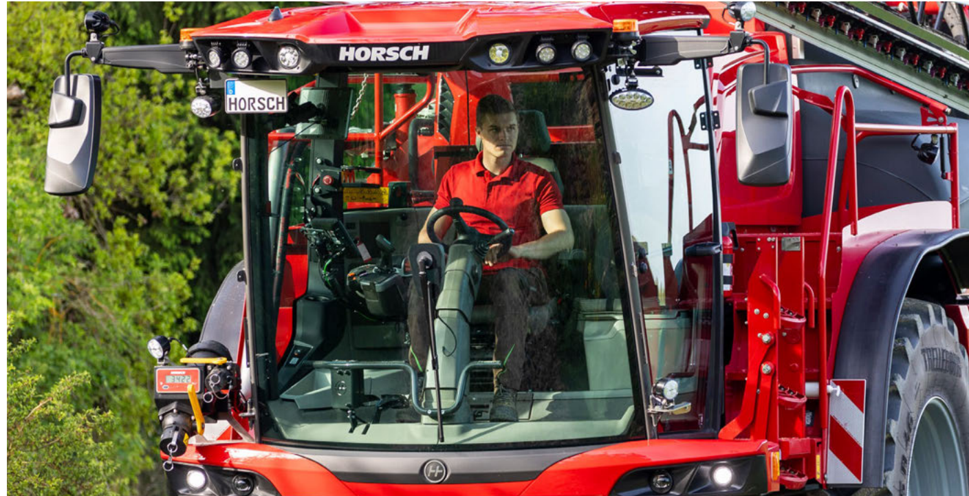
Cabin with large glass surfaces for optimum circumferential visibility
