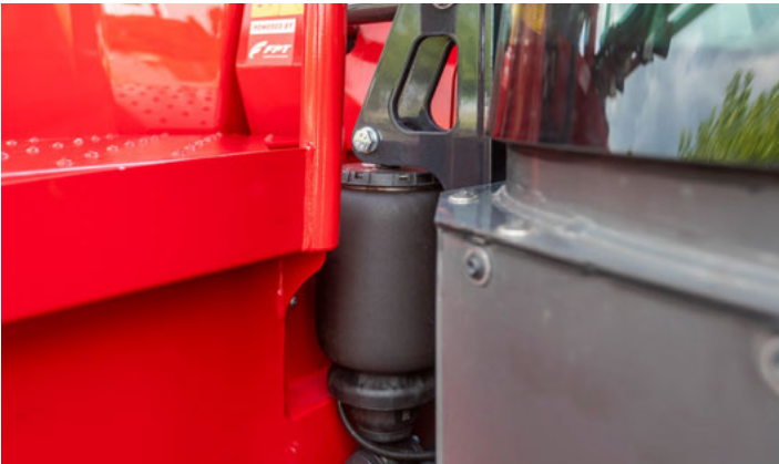
Pneumatic 4-point cabin suspension
