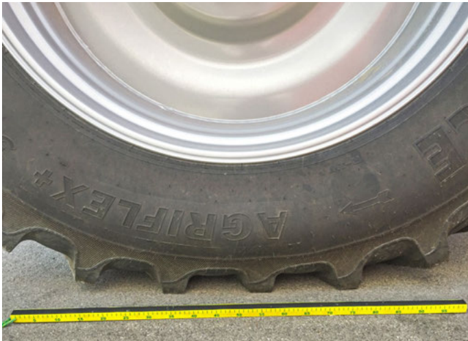
ATP Control – smooth running with a tire pressure of 33 PSI
