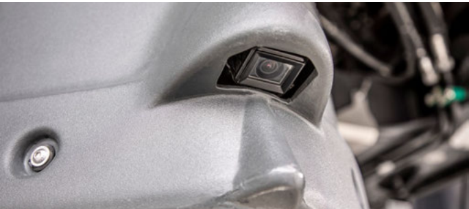
Camera integrated into the wheel housing
