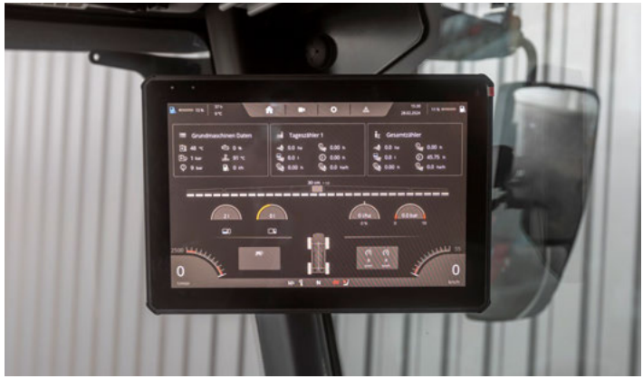
Standard 12" A-column display with freely assignable display
