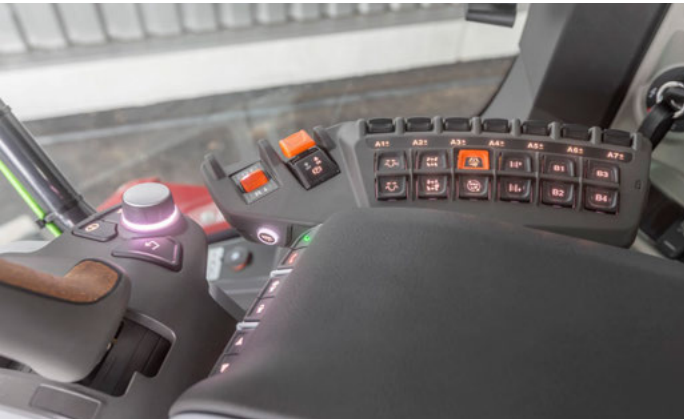
Comfortable operation of the functions compactly integrated into the armrest
