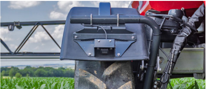
Camera lens with a view of the right front wheel
