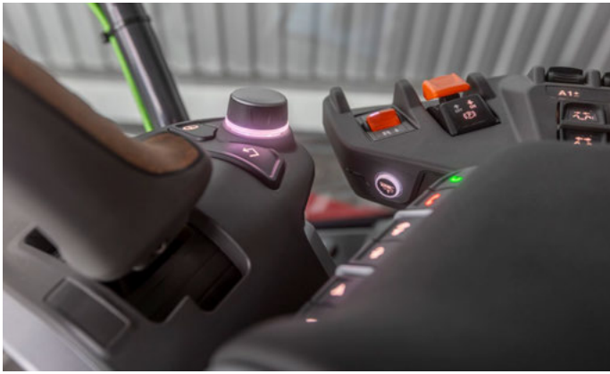
Safe operation of the A-column display: rotary/push functions
