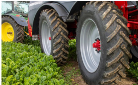
High maneuverability and stability with up to 35" of ground clearance
