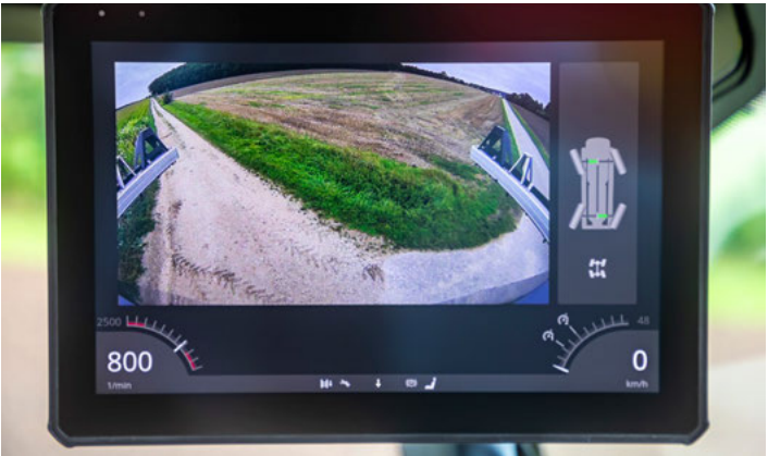
High-resolution, automatic display of the rearview camera in the A-column display
