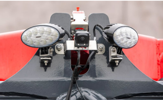
Rear view camera for monitoring the area behind the vehicle
