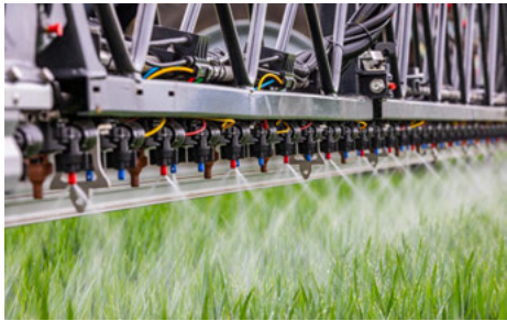
10'' nozzle layout: more nozzles more possibilities e.g. 3D application
