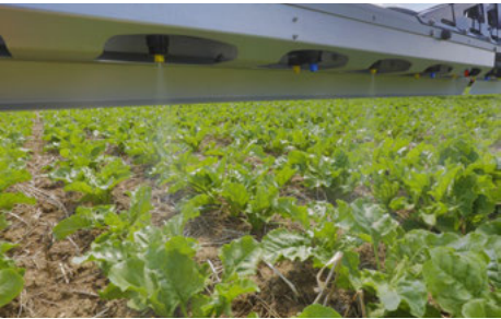
Band spraying is also no problem for a 10'' spacing
