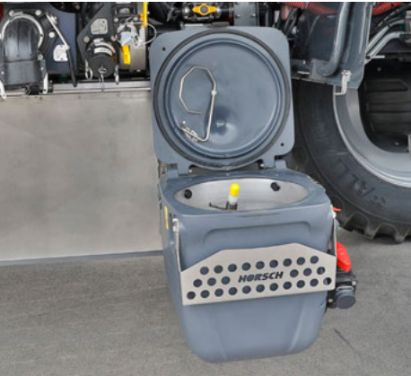
14 gal stainless steel induction hopper incl. additional shock nozzle
