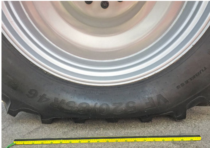
ATP Control – increased contact area at 14 psi tire pressure
