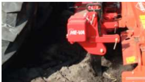
Adjustable height of rear cross points.
