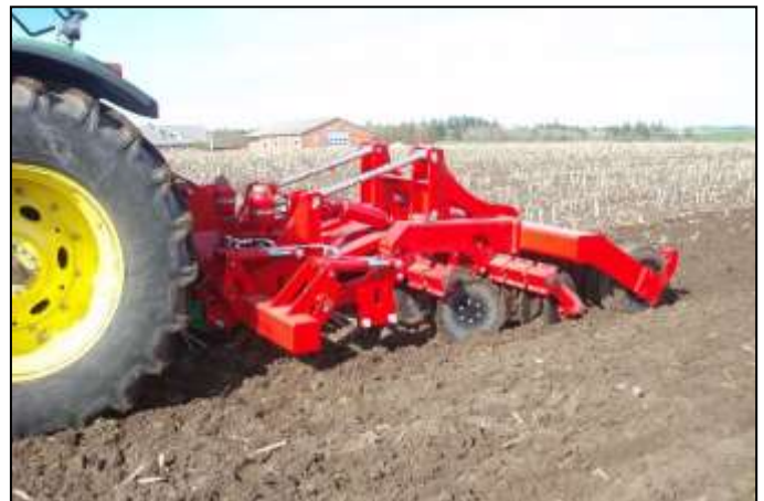
Combi-Disc with the tines in max. working depth, ensuring a soil loosening, cultivation and a consolidation.
