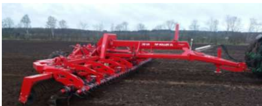
12,30 m Tip-Roller XL with Cambridge rings & 2-row Spring-Board
