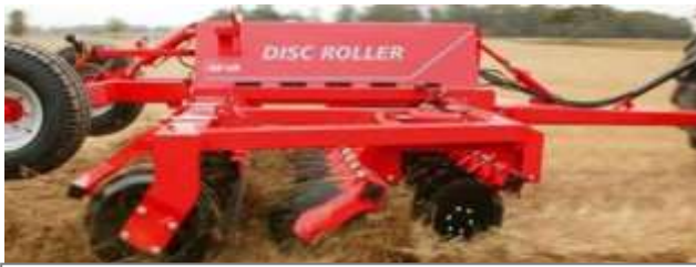
5,00 m w/V-Profile ring & material-damper guard.
