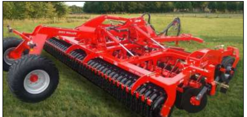
6.50 m Disc-Roller Contour w/V-Profile roller, material-damper guard, pivoting support wheels and two point pivoting crossbar.
