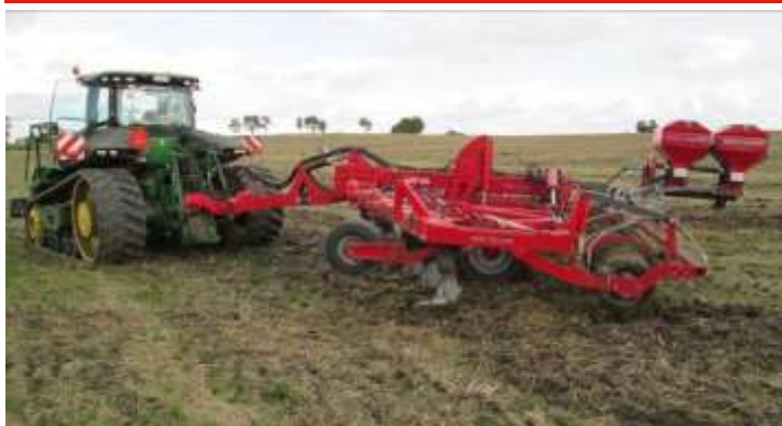
7,00 m with hydr folding, 13 tines, V-profile roller & hydr. auto-release system.
