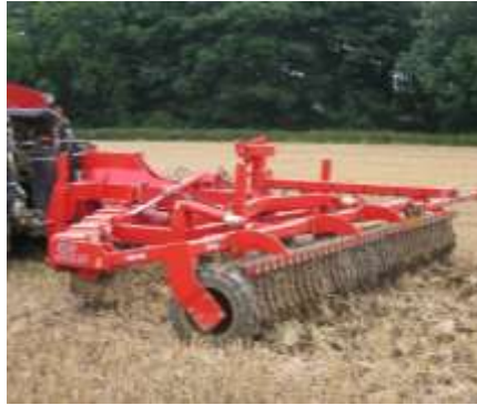
4,00 m Sub-Tiller w/hydr. folding, 7 tines, V-profile roller & Quick-Push stone protection.
