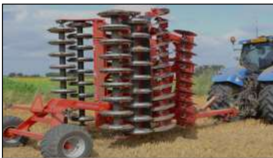
5.50 m Disc-Roller Contour w/Twin V-Profile roller and material-damper guard.
