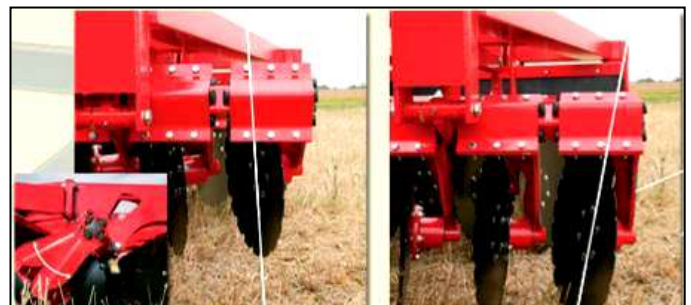
Standard equipment on all models: Adjustable edge disc for retain soil on right side.
