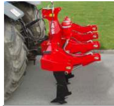
3,00 m. m/hydraulic auto-release system & 4 tines.
