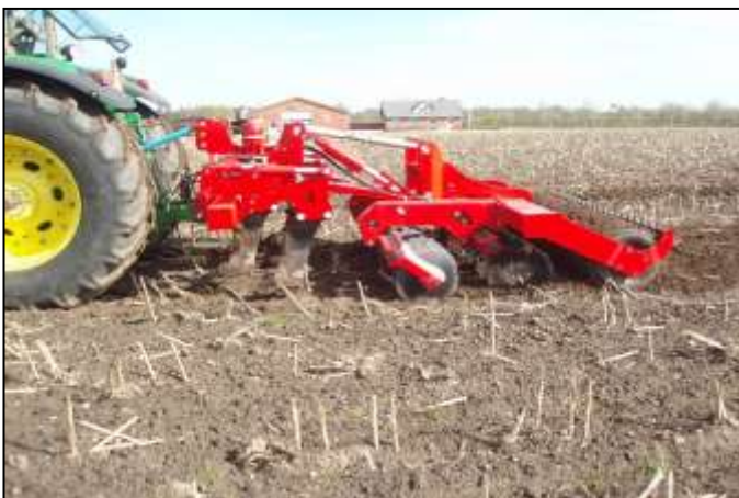
Combi-Disc with the tines lifted free from the soil, meaning that only the Disc-Roller's function is in work.
