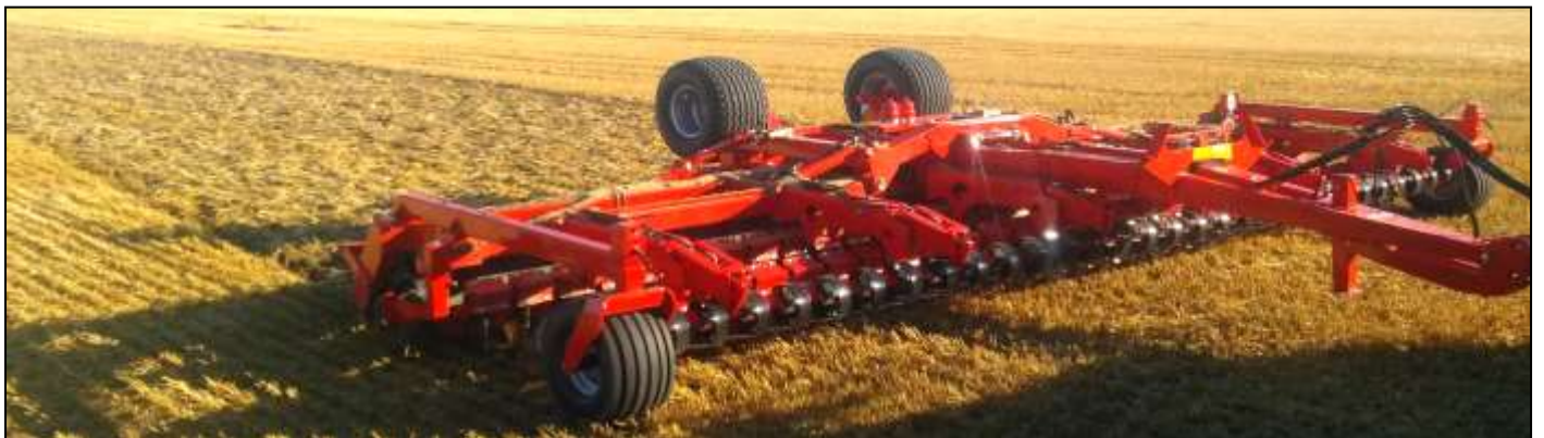
6.50 m Disc-Roller Contour w/V-Profile roller, material-damper guard, pivoting support wheels and two point pivoting crossbar.
