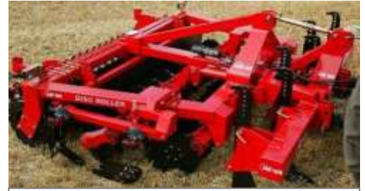
3,00 m trailed Combi-Tiller MKI with 3,00 m trailed Disc-Roller Contour.
