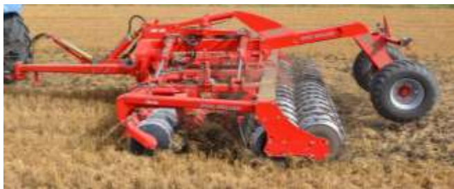
8,00 m Disc-Roller Contour with V-Profilroller and support wheels.
