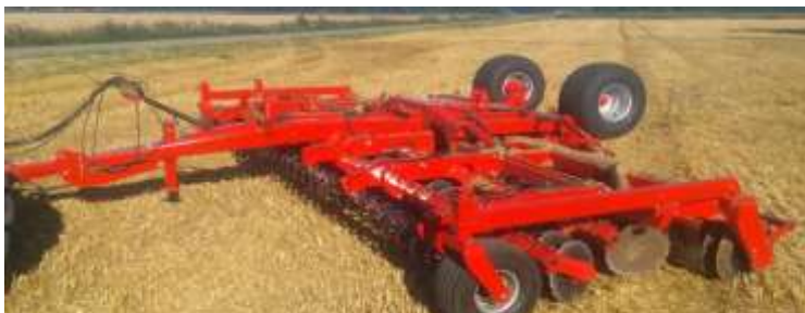
5,50 m Disc-Roller Contour w/Twin V-Profilroller & material damper guard
