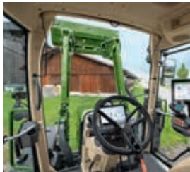
Panoramic front window with 77° vision for a full view upwards and over the wheel fenders.
