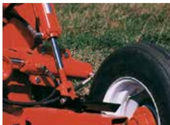
Hydraulic raising or lowering Of the rear wheels to quickly pass from transport position to working position.
