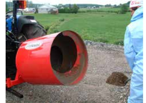
Spiral vane for mixing or emptying.
