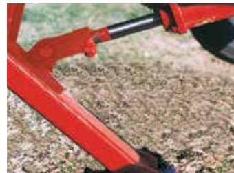
Front hydraulic jack Making hitching easy.
