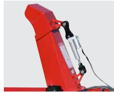
Electric actuator (Puma-48 to Puma-72)
