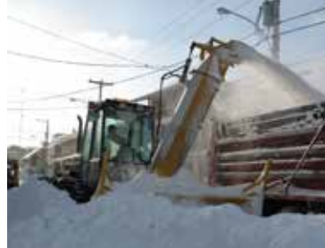
INDUSTRIAL, FULL FLIGHT AUGER
