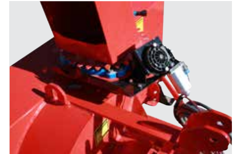
Electric motor (Puma-48 to Puma-72)
