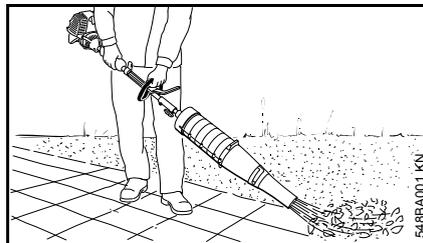
Always hold the unit firmly with both hands on the handles. Right hand on control handle, left hand on loop handle on the shaft, even if you are left-handed. Wrap your fingers and thumbs around the handles.
