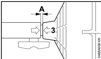
When correctly mounted, the intake screen (3) must be flush with the coupling sleeve (gap 'A' no more than 5 mm).
