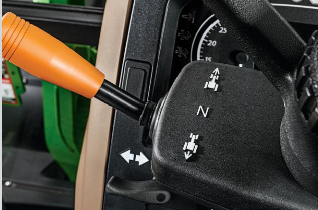
The PowrReverser helps you smoothly change directions without needing to change gears or touch the clutch ... a must have for fast loader work.
