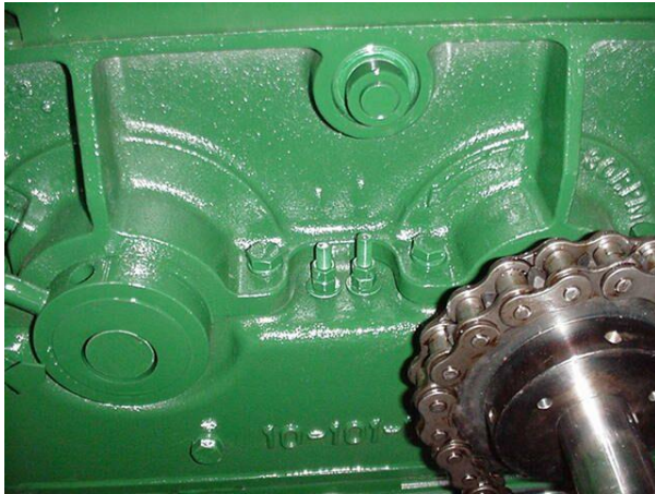
Figure 149 - Roll Scraper Adjustment Bolts
