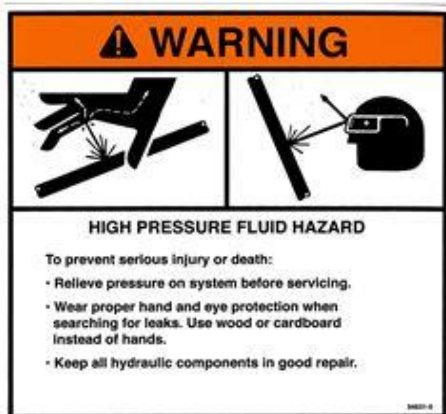
8. WARNING –High Pressure Fluid Hazard (346310)
