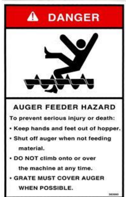
4. DANGER – Auger Feeder Hazard (383990)
