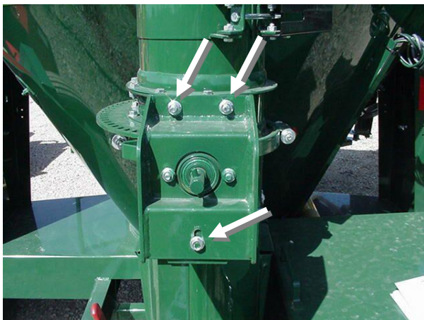
Figure 150 - Manual Unloading Auger Swing Crank Adjustment
