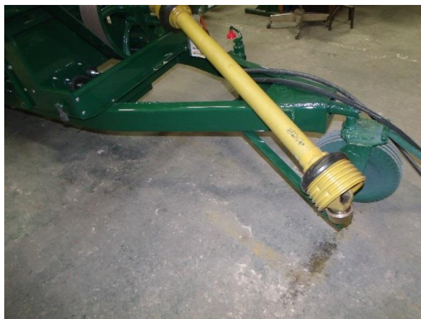
Figure 66 - PTO Driveline (Shield Removed For Clarity).
