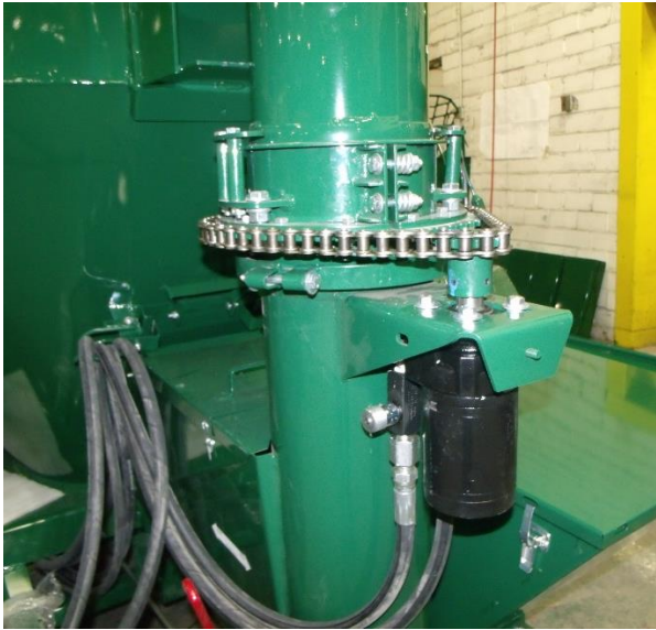
Figure 153 - Hydraulic Swing Adjustment (Shields Removed For Clarity).
