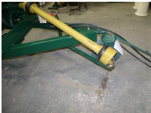
Figure 162 - PTO Driveline (Shield Removed For Clarity).
