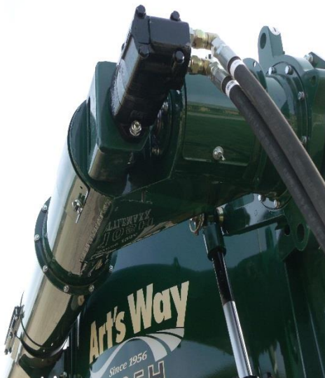
Figure 156 - Upper Discharge Motor (Unload)
