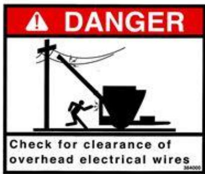
5. DANGER - Electrocutation Hazard (384000)
