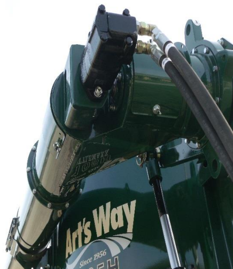
Figure 55 - Upper Discharge Motor (Unload)
