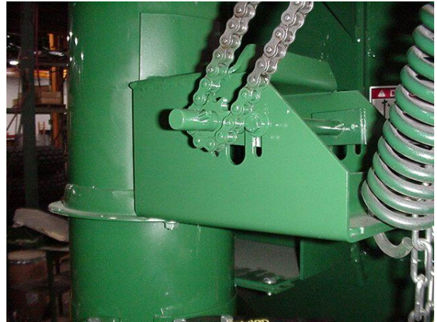
Figure 53 - Crank Shaft Chain Adjustment Bolts
