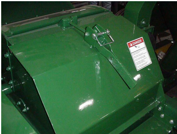
Figure 20 - Locking Pin and Latch on Hammermill Door (26 Inch Hammermill Shown).
