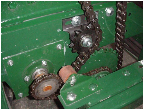
Figure 181 – Sprocket And Chain Alignment
