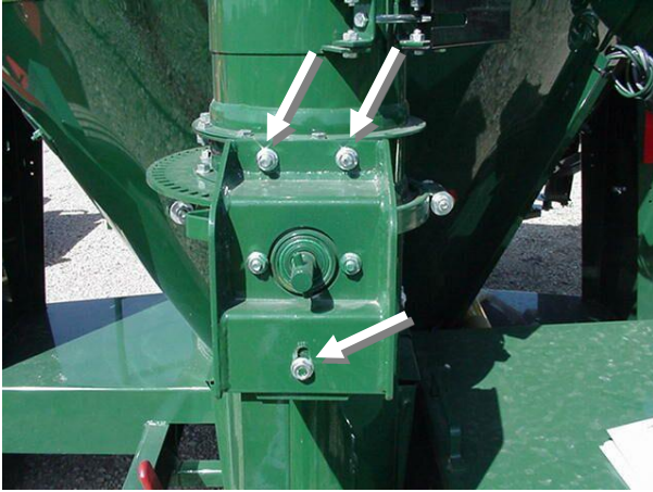
Figure 51 - Manual Unloading Auger Swing Crank Adjustment
