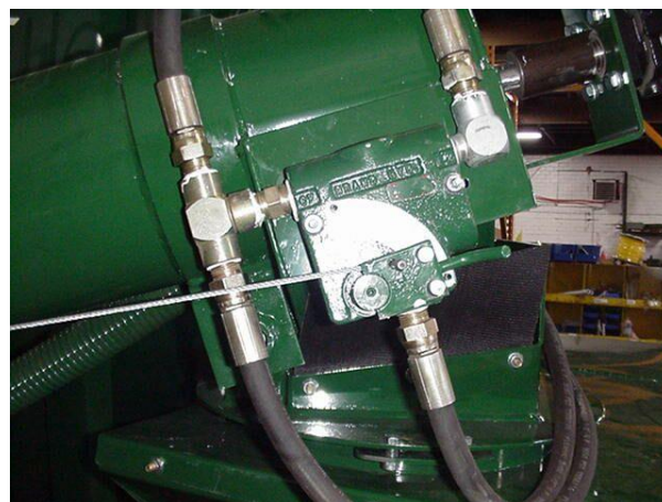
Figure 141 - Auger Feeder Flow Control Valve (Shown In "ON" Position).
