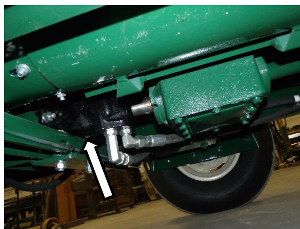
Figure 57 - Lower Discharge Motor (First Section)
