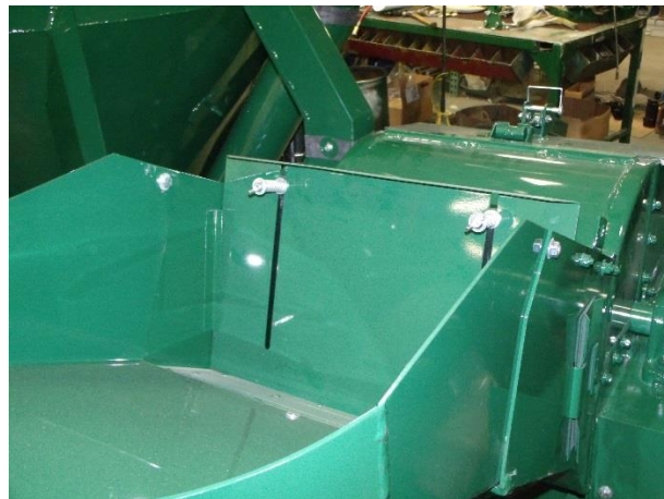
Figure 17 - Feed Gate At Throat Of The Hammermill.
