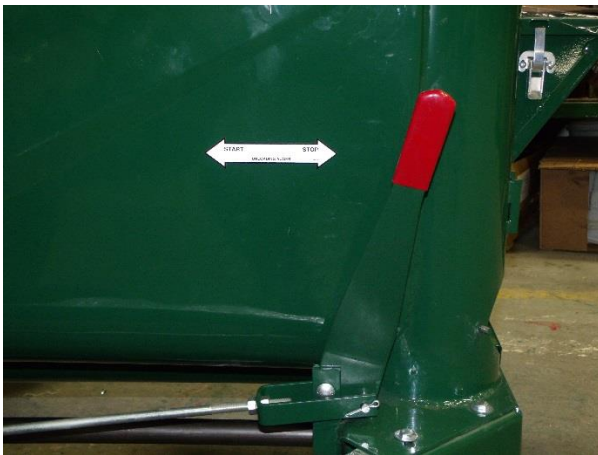
Figure 29 - Unloading Clutch Operation.
