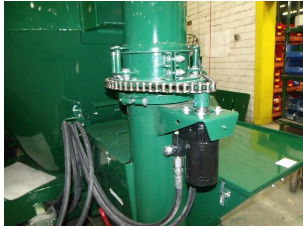
Figure 60 - Hydraulic Swing Adjustment (Shields Removed For Clarity).
