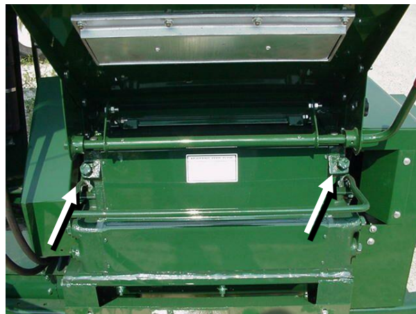
Figure 164 - Grain Control Gate Lubrication (2 Zerks and Slide Guides).
