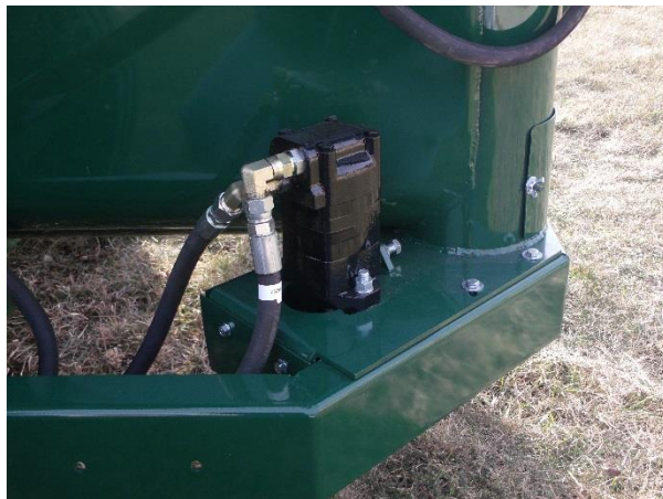
Figure 157 - Middle Discharge Motor (Vertical)
