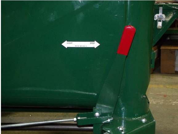
Figure 131 - Unloading Clutch Operation.
