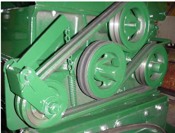
Figure 166 – Rollermill Belt Drive
