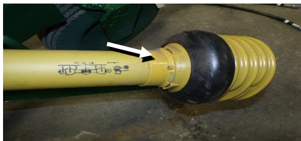
Figure 163 - Plastic Shaft Bearings (See Arrow).
