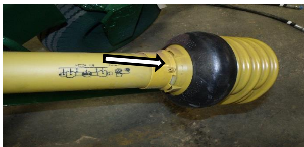
Figure 67 - Plastic Shaft Bearings (See Arrow).
