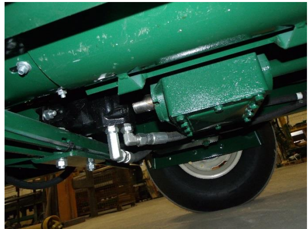
Figure 158 - Lower Discharge Motor (First Section)
