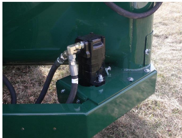
Figure 56 - Middle Discharge Motor (Vertical)
