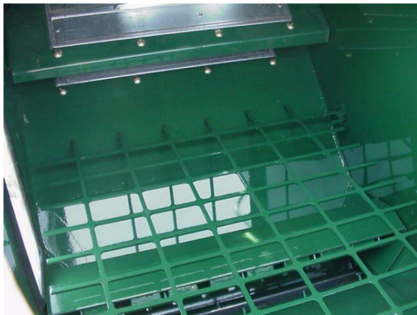
Figure 148 - Removing Magnet To Check Roll Spacing.
