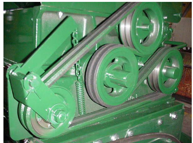
Figure 146 - Drive Chain Adjustment (Shields Removed For Clarity).
