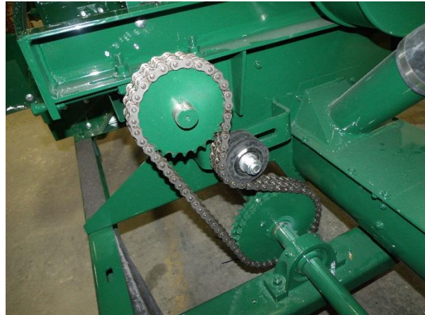
Figure 44 - Drive Chain Adjustment (Shields Removed For Clarity).
