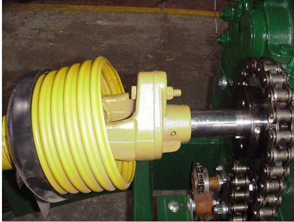
Figure 118 - PTO Driveline Shear Clutch
