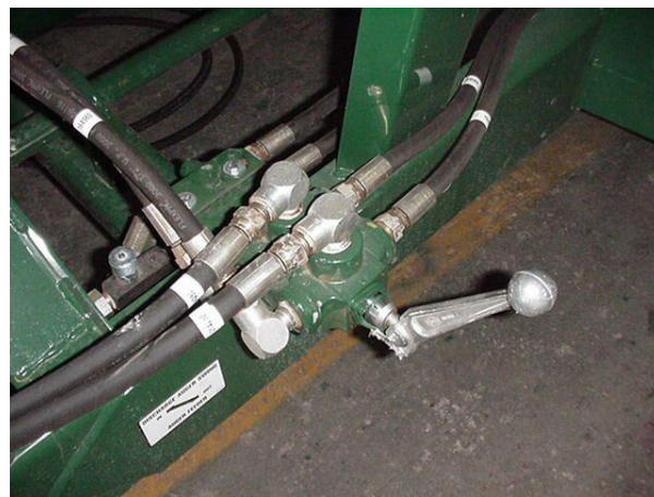
Figure 142 - Hydraulic Auger Feeder Selector Valve Lever Is In The Out Position - Auger Feeder).
