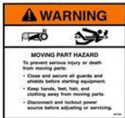
9. WARNING – Moving Part Hazard (467450)
