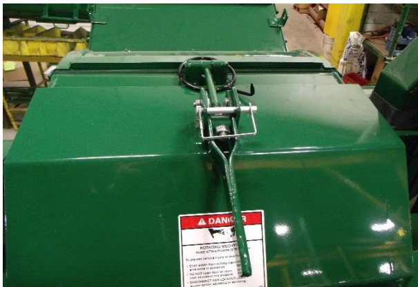
Figure 8 - Screen Hook Storage.
