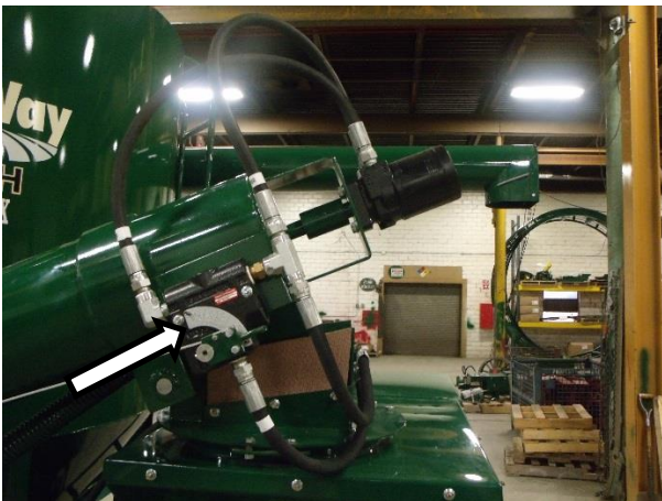
Figure 40 - Hydraulic Auger Feeder Control. (See Arrow)
