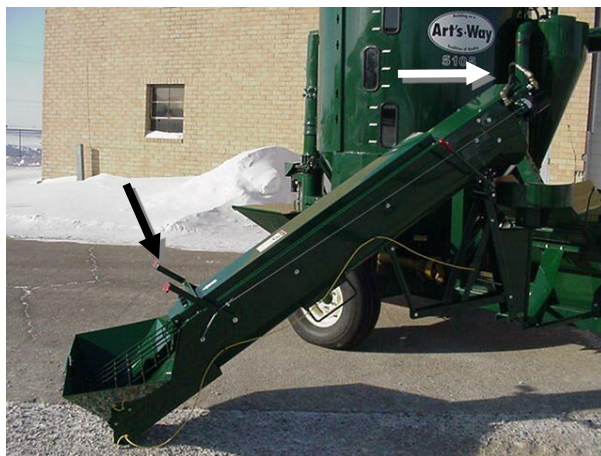
Figure 39 - Hydraulic auger feeder controls. (See arrows)
