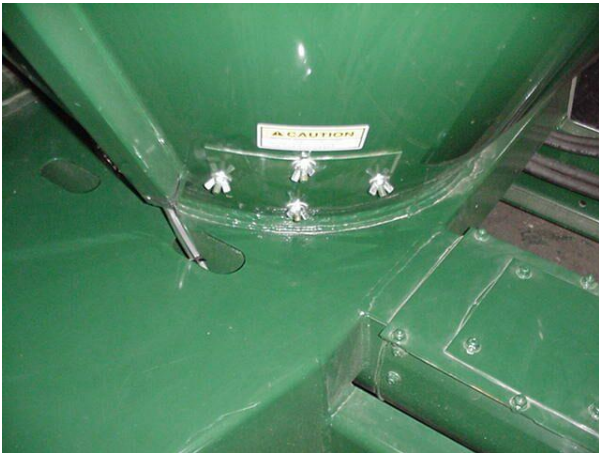
Figure 123 - Tank Cone Clean-Out Door On Right-Hand Side.
