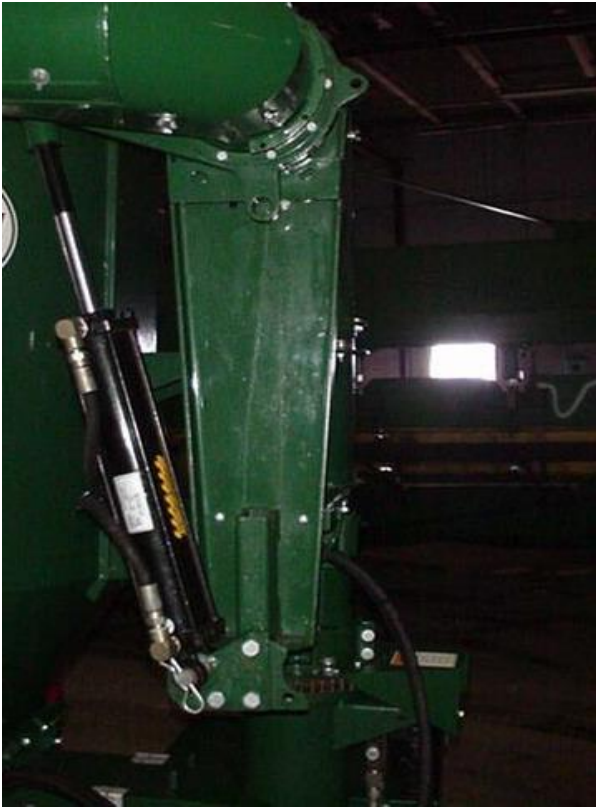
Figure 58 - Discharge Auger Lift Cylinder Adjustment.
