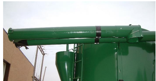
Figure 32 - Folding Auger Extension. (6' Extension shown)
