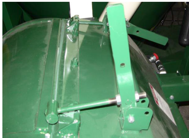
Figure 23 - Hammermill Door Pressure
