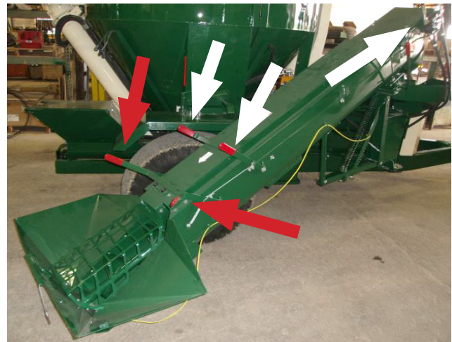
Figure 16 - Hydraulic Auger Feeder controls (shown in off position): Throttle controls (white arrows) and Emergency Shutoff (red arrows)
