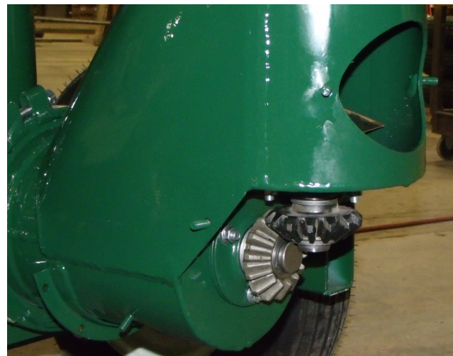
Figure 8 - Discharge Joint Location
