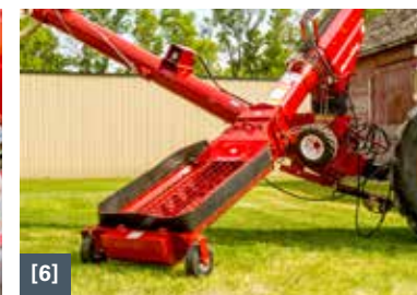
[1] Accessible operating levers [2] Low profile hopper tilts to swing intake into position [3] Posi-Track drive system [4] Hydraulic winch [5] Mounting ring; to fit-up to BackSaver augers [6] Fully retracts
