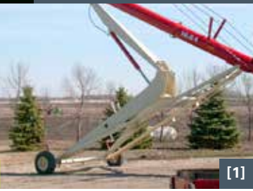
[1] Undercarriage, 10" model shown [2] Adjustable light [3] Gearbox [4] Dual spool valve (option) [5] Auger steer (option)
