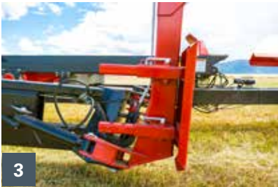
[1] Two hydraulic motors power the bale pusher [2] Rear unloading forks [3] Reinforced carrier arm [4] Pusher chain [5] Hydraulics
