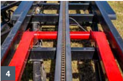
[1] Two hydraulic motors power the bale pusher [2] Rear unloading forks [3] Reinforced carrier arm [4] Pusher chain [5] Hydraulics
