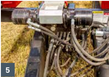
[1] Two hydraulic motors power the bale pusher [2] Rear unloading forks [3] Reinforced carrier arm [4] Pusher chain [5] Hydraulics
