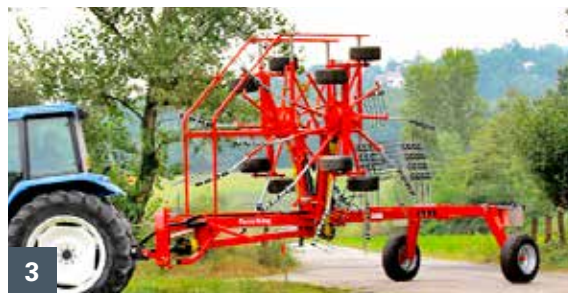
[1] Cardan shaft. [2] Complete cleaning of the ground thanks to the intersecting arms. [3] Steering system allows great maneuverability. [4] Full intersection of arms.
