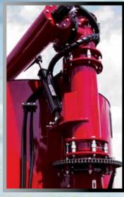
An adjustable slip slutch on the auger rotation provides protection if foreign objects are encountered.
