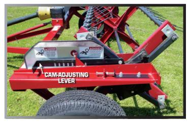
The angle of the rubber mounted teeth can be changed easily just by moving the handy lever to adjust the cam. Tedding will allow air to move through your hay for much faster drying, assuring uniform curing and higher quality hay.
