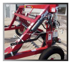
The **hand crank** (1) is for tedder reel height adjustment. The cam lever (2) is used to adjust the aggressiveness of the tedder teeth for a fluffier windrow.
