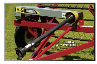
A **screw type link** (below the PTO Shaft) allows for handy and easy height adjustment. Cut hay that has been rained on can be tedded to speed up drying and avoid spoiled hay.
