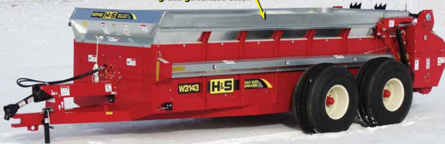
MODEL W3143 430 Bushel, Struck level 275 cu. ft.
