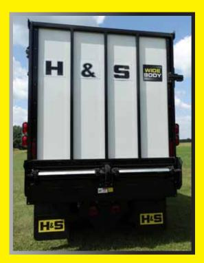
Fiberglass reinforced plywood (FRP) side Wide Body boxes are available in 22', 24' and 26' lengths.
