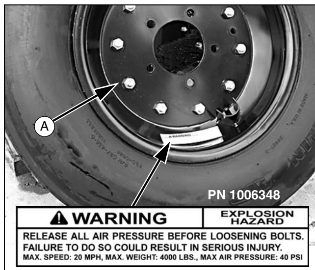
Figure 23. Split Rim Tire Servicing
