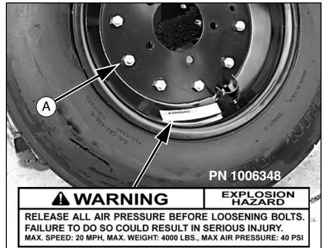
Figure 8. Split Rim Tire Servicing
