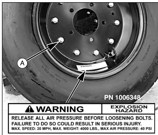
Figure 23. Split Rim Tire Servicing
