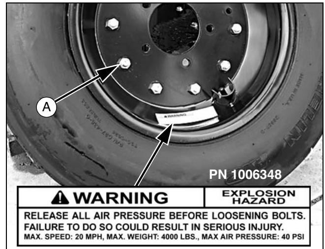
Figure 8. Split Rim Tire Servicing
